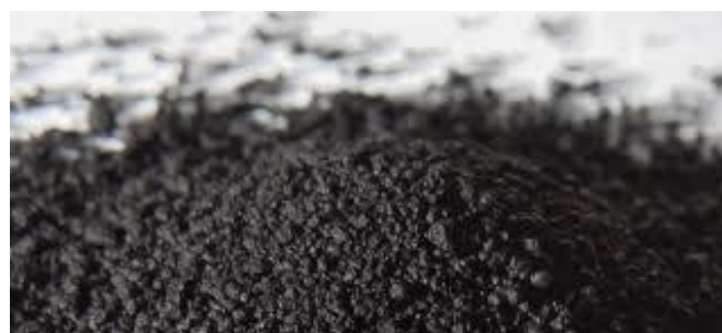
Carbon black comes in various subtypes such as acetylene black, channel black, lamp black and thermal black
