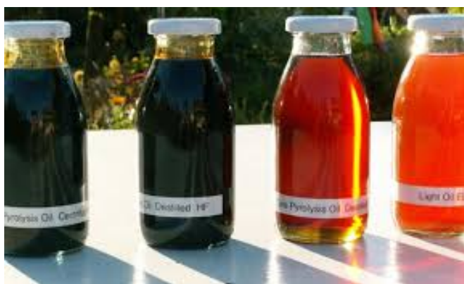
Sample of pyrolysis oil which is a by-product that can be used as fuel
