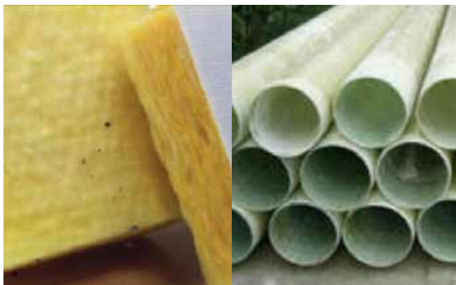
Sample of fibreglass pipes to the left and insulation panels to the right using fibreglass
